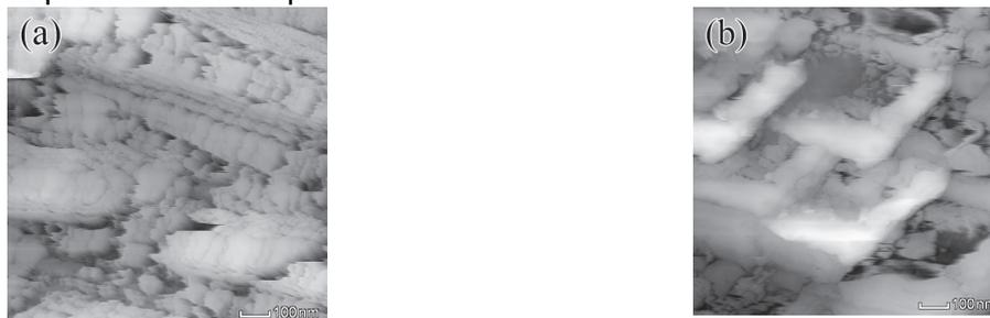
**Fig. 2.** (a) –STM image of Ni surface before heating (b) – STM image of graphene nanobubbles at the same place after heating
