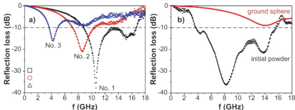
Figure 1. The frequency dependencies of the reflection losses (a) – for samples No. 1, No. 2, No. 3 and (b) – for samples from not separated powders (initial and ground spheres). Measurements are carried out in “reflection” mode using short-circuited load.
