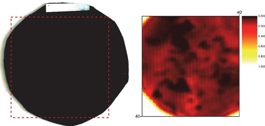
Figure 1 - Composite material based on polymethyl methacrylate and MWCNT (left) and THz image (right).
