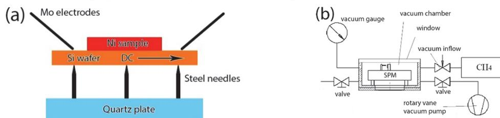
**Fig. 1.** (a) –scheme of the sample holder with embedded heating system; (b) – scheme of the CVD system with embedded STM
