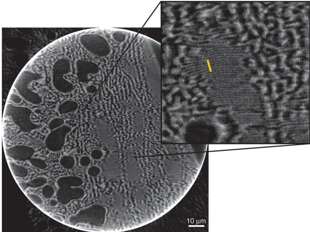
Fig. 1. Reconstructed tomogram slice of Al-Al<sub>2</sub>Cu eutectic microstructure.
