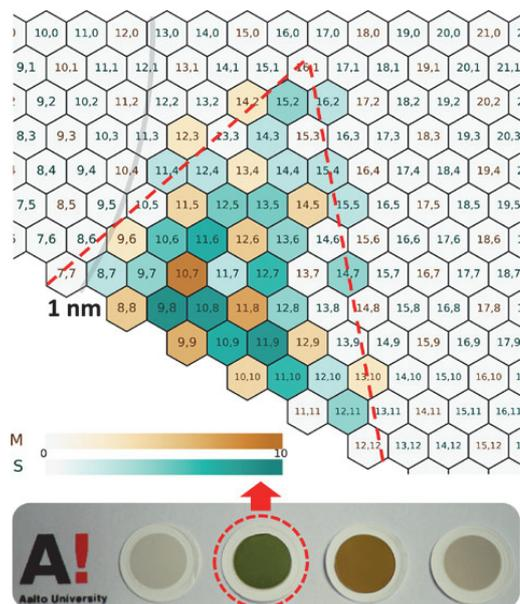
**Figure 1.** (n,m) distribution of the green SWNTs and photos of the SWNT thin films synthesized at 850 oC. with 0 %, 0.25 %(green), 0.37 % (brown) and 0.5 % of added CO<sub>2</sub>.
