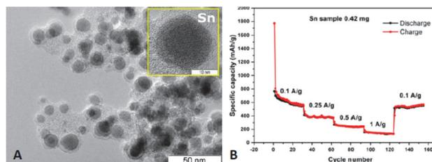
**Figure 1:** A – TEM image of the Sn/C composite; B – charge-discharge cycling performance of the Sn/C composite.
