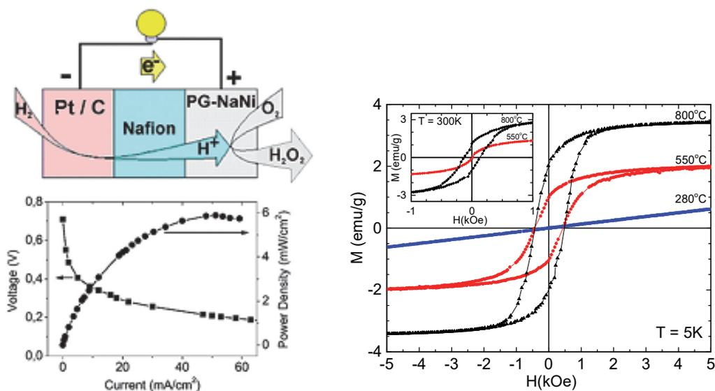
The representation (top left) of the H<sub>2</sub>/O<sub>2</sub> Proton Exchange Membrane Fuel Cell and polarization and power density curves (bottom left) with the catalyst from complex of pectin polygalacturonates with sodium nickel (PG-NaNi) (annealed at 90 °C) at the cathode and commercial Pt/C catalyst at the anode.
