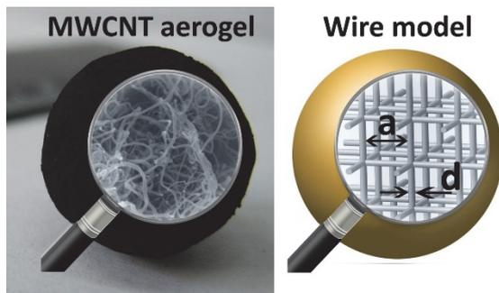
Figure 1. A spherical particle of MWCNT aerogel of 4.5 mm (left, the inserted in the form of lens presents scanning electron microscopy image of tangled nanotubes similar to those described in [1,2]) and an equivalent wire ball (right, where  $a$  is lattice parameter and  $d$  is nanowire diameter).
