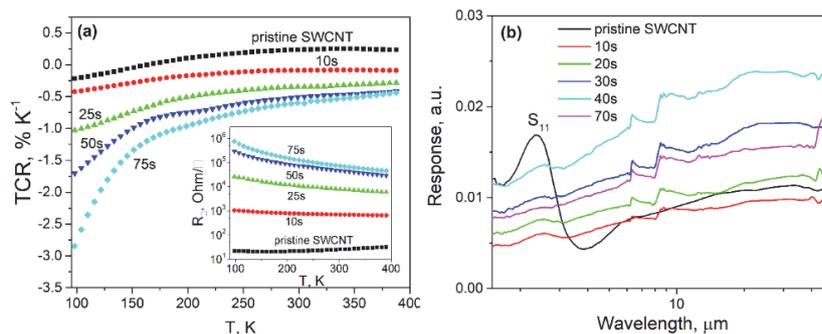
**Fig.1** The plasma treatment effect on TCR of SWCNT films and bolometers response (a) TCR of pristine SWCNT films and the ones treated in oxygen plasma at different exposure time, inset: temperature dependence of film sheet resistance. (b) Spectral characteristics of bolometric samples made of 100 nm thick free-standing SWCNT film, pristine and oxygen plasma treated with different time of treatment.
