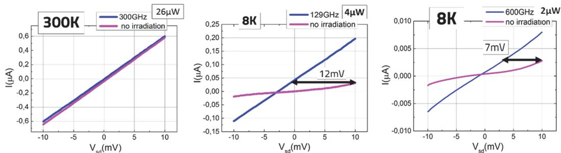
**Figure 1.** IV-curves for device type I at different temperatures (300K, 77K, 8K) measured in two conditions: with and without radiation. The response voltage is shown with the arrows.
