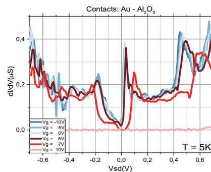
Figure 2:  $dI/dV$  curves of one of our SWCNT obtained at different values of the gate voltage.
