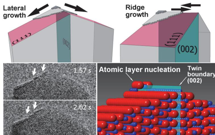
Fig. 1. *In situ* TEM observation of CuO nanowire growth [1].
