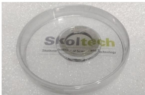
**Figure 1:** The free-standing thin film of single-walled carbon nanotubes.
