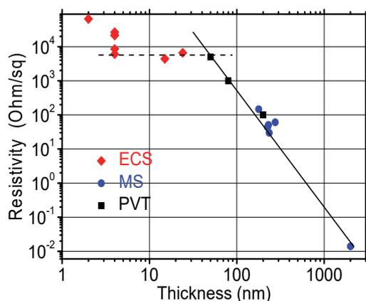
**Fig. 1.** The dependence of the Bi<sub>2</sub>Se<sub>3</sub> films resistivity on their thickness.
