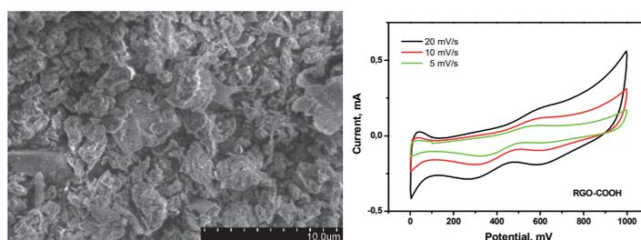
**Figure 1.** SEM image of RGO-COOH and CV curves of carboxylated graphite oxide, measured at the scan rates of 5, 10 and 20 mV/s in 1M H<sub>2</sub>SO<sub>4</sub> in the three-electrode cell.
