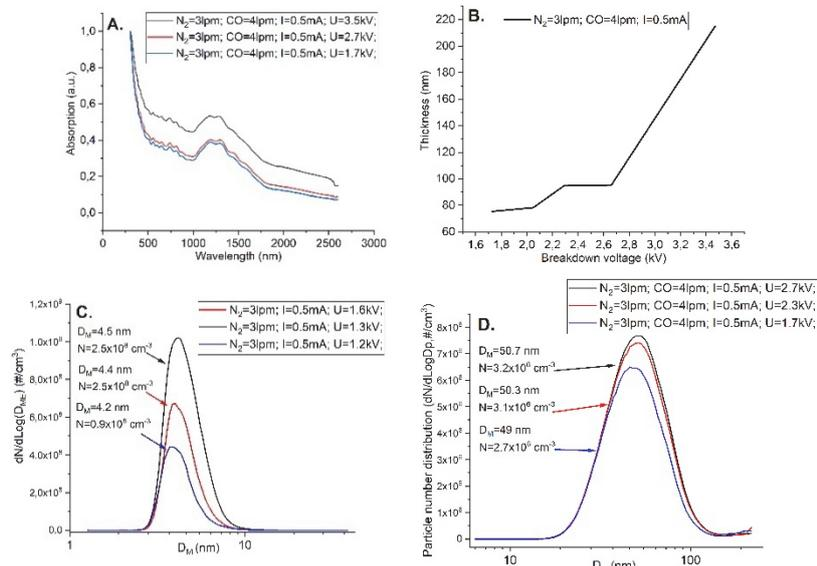
**Figure 1.** Influence of a breakdown voltage of spark-discharge generator on: (A) - optical spectra of SWCNTs; (B) – thickness of films (1cm filter, 30min collection time); (C)- diameter distribution of catalyst particles; (D) - mobility diameter distribution of single-walled carbon nanotubes.
