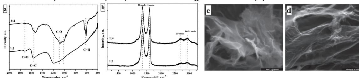
Figure 1: FTIR (a), Raman (b) and SEM images of rGO obtained using 1.6 g (c) and 0.5 g (d) of hydrazinium sulphate.
